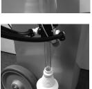
5. Working the adjustable ball joints of the nozzle assembly-mounting arm, point the nozzle straight down. Then move the nozzle assembly to the side of the HaloFogger EXT, locating the assembly above the waste bottle.
