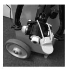
1. Attach the ends of the HaloFogger EXT hoses to their respective air and fluid receptacles on the fogger. (See icons on fittings.)
