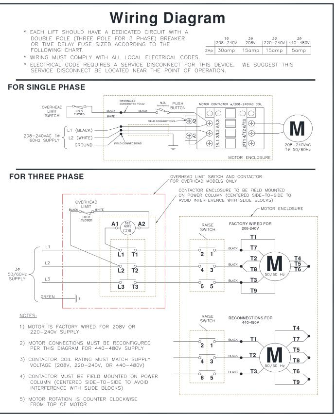
Fig. 12 – Electrical Wiring Diagram
