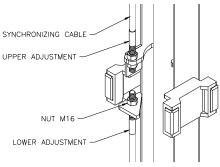
Fig. 5 – Synchronizing Cables
