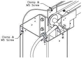
Fig. 9 – Lock Cable Routing
